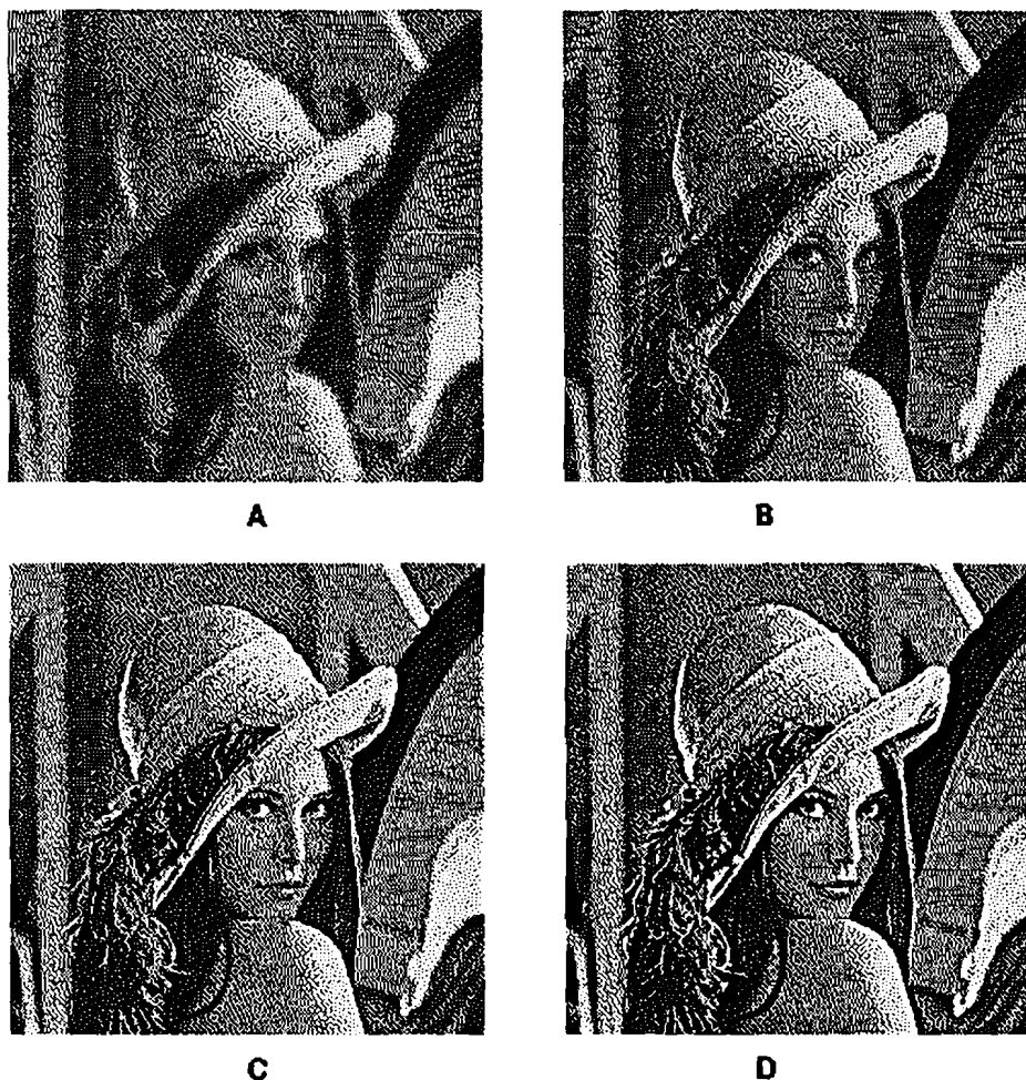
Figure 3.24: Error diffusion with the input image as threshold modulation function, (A) \kappa = 0 , (B) \kappa = 1 , (C) \kappa = 2 and (D) \kappa = 3 .
