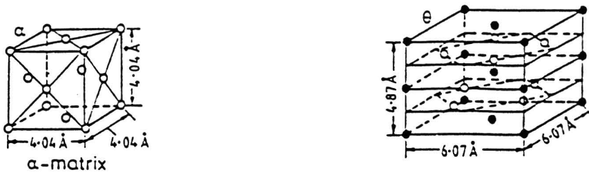
- Figure 24 - The structure of the fcc ( \alpha ) and the \text{Al}_2\text{Cu} \theta phase. The dark atoms are Cu, white Al [A4].
