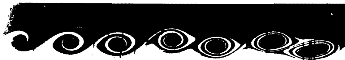
Figure 8. Roll-up of vortices. f_r \approx f_n . R < 1 . (Ho and Huerre, 1984)
