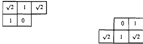
Fig. 2.6 : The masks W (left) and W' of the CDT for calculation of the euclidian chamfer distance.
