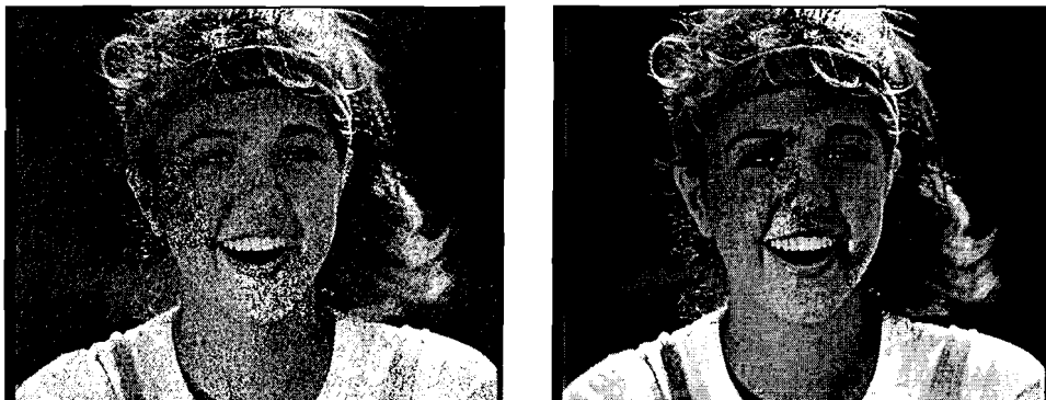
Figure 1.1: Teeny with a PSNR of 20 dB and noiseless Teeny
