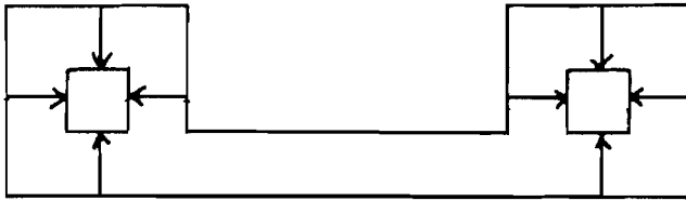
Fig. 6.2. A shrink operation on mask-data is a local operation and can let some areas disappear.
