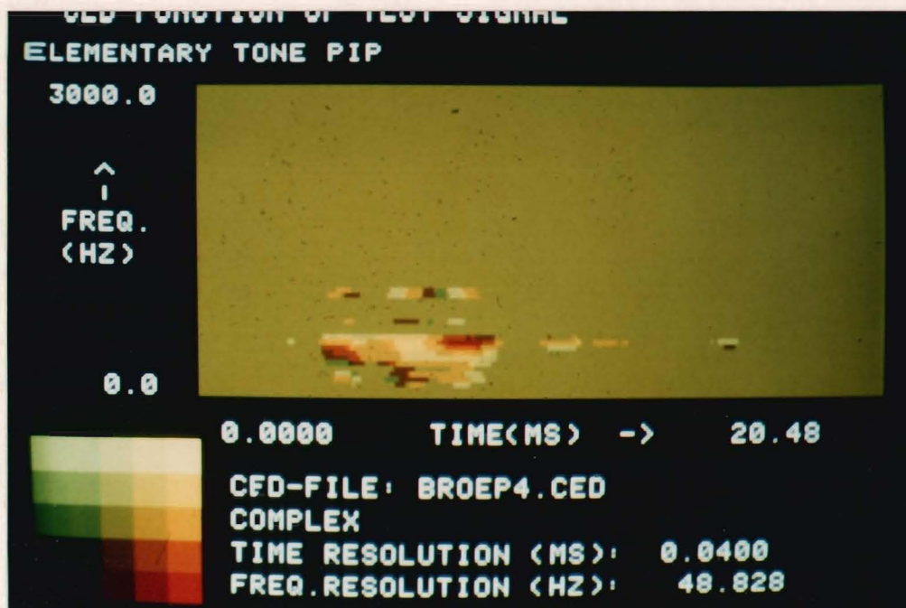
Fig. 4.49.a. The CoSTID-function of an element from a B-call of the frog Rana temporaria with rectangular coding.
