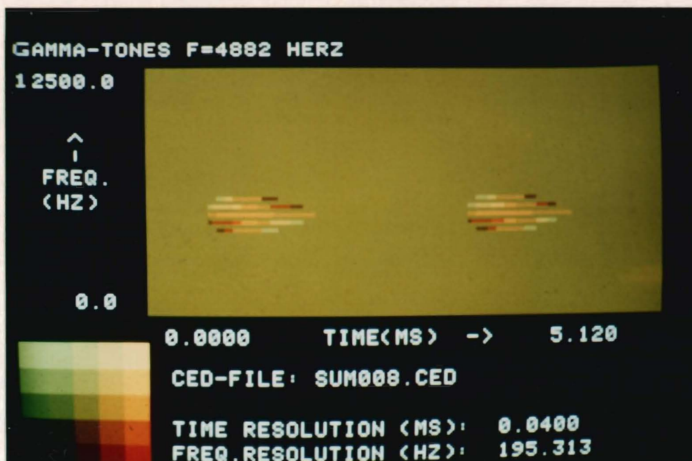
Fig. 4.18.a. The COSTID-function of two time shifted gamma-tones with rectangular coding.
