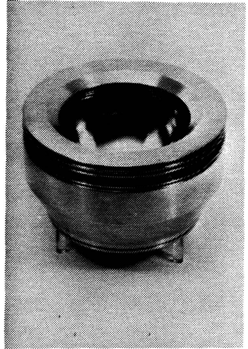
Fig. 3.4.a,b. The toroidal analyzer segments and the elements of the zoomlens.
