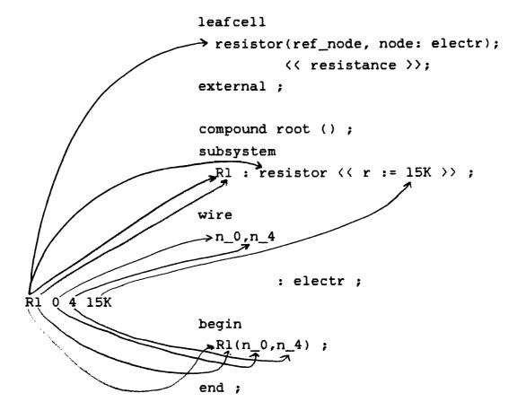
Figure 6.1 Translation of a circuit element
