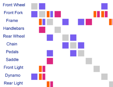
Figure 1: Example DSM of a bicycle. Purple matrix entries indicate a mechanical, moving interface between components; pink indicates a rigid mechanical interface; and orange an electrical interface. Some pairs of components have multiple types of dependencies between them. For example, there is a mechanical, moving connection between Front Fork and Frame, but also an electrical one: The Front Fork is able to rotate relative to the Frame, to allow steering. Since the Dynamo of the bike in this example is mounted on the Front Fork, current from the Dynamo travels via the Front Fork to the frame to reach the Rear Light, resulting in an electrical connection between Frame and Front Fork as well.
