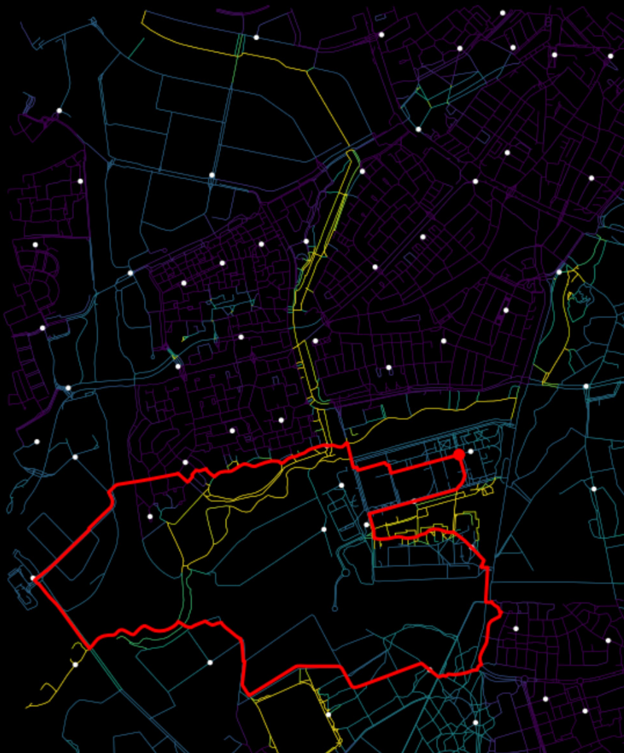
Figure 10.3: The result of the second stage. The colors on the road network contain the score of each route segment, based on the user's preferences. The red line shows a suggested route. The dots were used to determine a rough path on the first pass.
