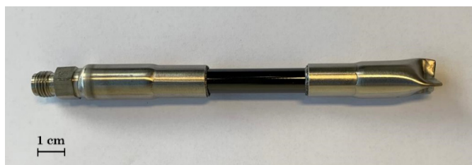
Figure 5.2. Carbon molecular sieve membrane sealed with a dead end metallic tube from one side, and a metallic tube with a Swagelok connection on the other side.
