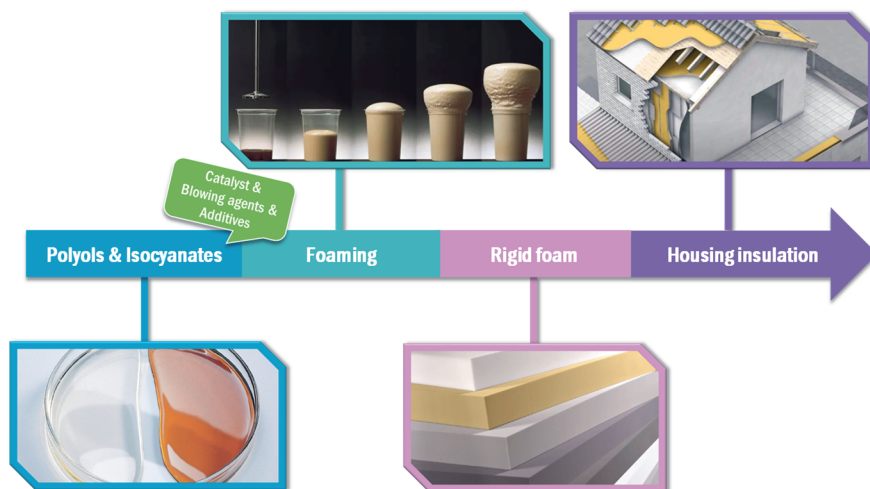
Figure 1-3. From the one-pot synthesis to construction applications of PIR-PU rigid foams. The isocyanates and polyols are reacted in molar ratio from 2:1 to 5:1 (index 200 to 500) with presence of trimerization catalysts, urethane catalysts, surfactants or other additives. After the foaming process, PIR rigid foams are obtained. These foams can be used in houses to provide good thermal insulation. Images obtained from BASF website.
