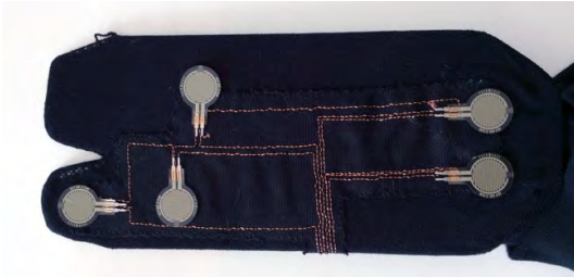
Figure 2. Inside of the sole of the second proof of concept. Conductive traces were embroidered on cotton fabric to allow for soldering the FSR sensors in fixed positions. The cotton was attached to an off-the-shelf hallux sock.
