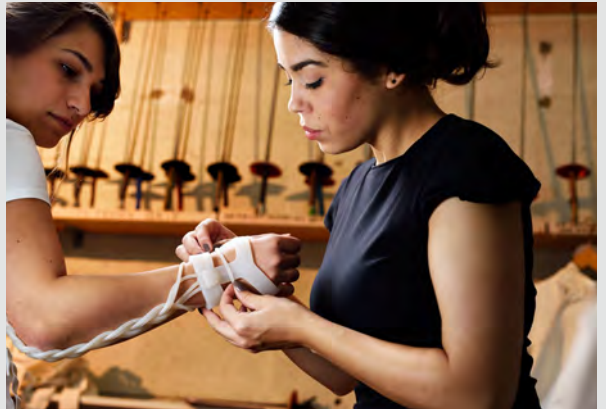
Fig. 11. Flow (2015). Bruna Goveia da Rocha. Flow is a wearable that includes six inflatable chambers that push against the body to cue fundamental joint movements of the wrist and forearm to foster learning physical activities, such as fencing. The integrated chambers and air ways in Flow operate as a material extension of the actuators responsible for the inflation, removing the air pumps from the area of actuation. Consequently, the wearable can be technically and materially sophisticated whilst remaining lightweight.
