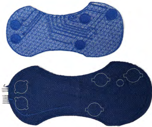
Figure 12. Size difference between research products 2 (top) and 7 (bottom). The relative distance between components was preserved while resizing the substrate shape.
