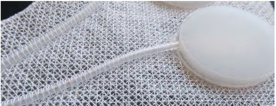
Figure 1. Detail of sample created in the project through a process of Exquisite Fabrication. The fabrication of this embroidery- based inflatable sample took four steps, done in three different machines: digital machine embroidery, a filament 3D printer and a custom Liquid Deposition Modeling (LDM) 3D printer. The steps were a) embroidering the substrate, b) 3D printing a mold on the embroidery, c) 3D printing the silicone and d) integrating the tubing through a couching stitch.
