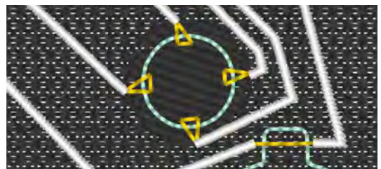
Figure 6. Detail of research product 7 showcasing part of the conductive traces under insulation zigzag stitch exposed and placeholders (blue markings) for attaching sensors.
