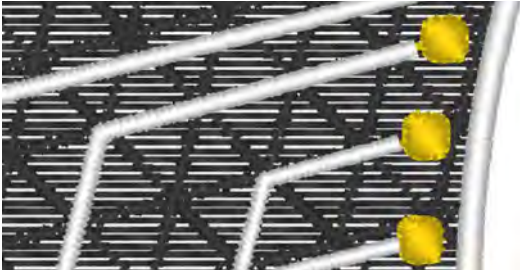
Figure 8. Detail of research product 3. The contact pads facilitated the temporary connection to electronics or multimeters through testing clips.
