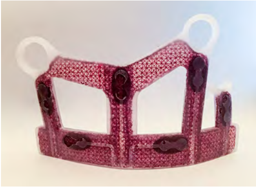
Figure 10. Sample 2.2 recreated Flow. The color changed significantly after casting, particularly on the denser areas.
