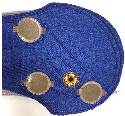
Figure 4. Detail of research product 7. The flexible PCB containing the accelerometer/gyroscope was designed to be embroidery friendly. The contact pads of the PCB were double-sided and wide to increase contact with conductive traces.
