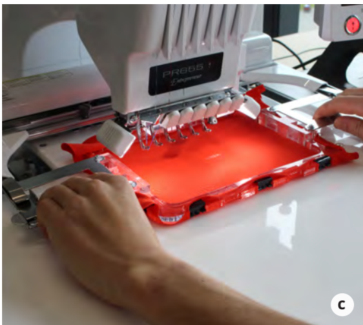
FIGURE 3 (a) Base-plate installed on a 3D printer; (b) Calibration; (c) embroidery frame mounted on an embroidery machine.
