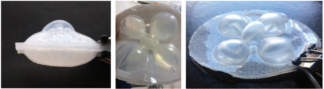
M1 Multi-state inflation a M2 Symmetrical inflation b M3 Unilateral inflation c
