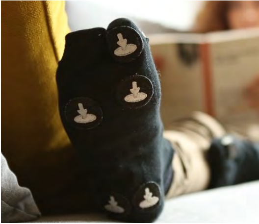
Figure 3. Sole of the second proof of concept. Embroidered pads were used to prevent the off-the-shelf pressure sensors from bending. Photo credit: Scott Delbressine
