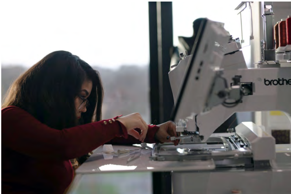
Figure E. Me placing needles at the Brother PR1050x digital embroidery machine in the Wearable Senses Lab
