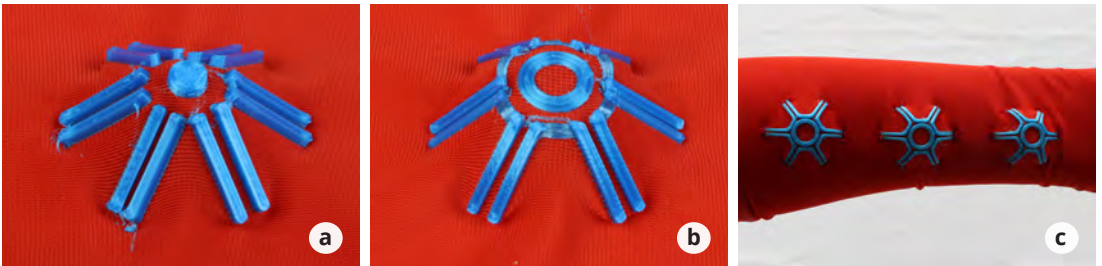
FIGURE 6 Isolated buttons: (a) star-like pattern; (b) a touch point added on the top; (c) 1x3 matrix of isolated buttons.
