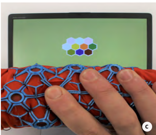
FIGURE 13 Connecting the FabriClick to a computer. (a) Connecting the embroidered circuitry to an Arduino using crimps; (b) Circuitry on the breadboard. (c) Results as an on-screen visualization of real-time signal processing.
