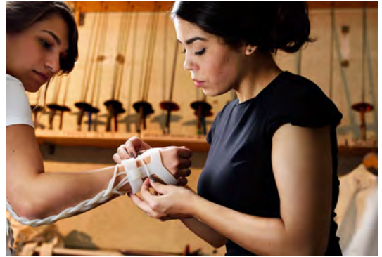
Figure 2. Flow (2015). Bruna Goveia da Rocha. Flow is a wearable that includes six inflatable chambers that push against the body to cue fundamental joint movements of the wrist and forearm to foster learning physical activities, such as fencing. The integrated chambers and air ways in Flow operate as a material extension of the actuators responsible for the inflation; removing the air pumps from the area of actuation. [10]
