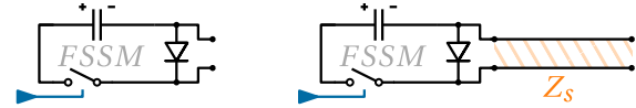
Fig. 4. FSSM schematic, consisting of MOSFET switch, HV capacitor, and bypass diode. FSSM without TL (left) and FSSM with TL (right) to set its characteristic impedance to Z_S .
