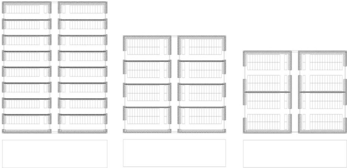
Figure 94. Plans of the archive, for 16, 8 and 4 vaults
