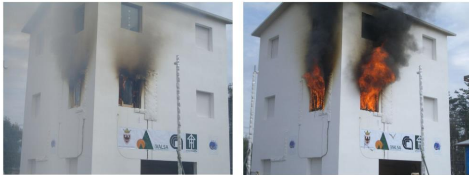
Figure 29. Fire development after about 32 minutes (left) and after 40 minutes (right) after ignition
