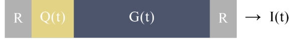
Figure 1: Schematic overview of the two section laser structure model. The optical cavity is formed by the two mirrors R, a loss section Q, and gain section G. The optical output is marked with I.
