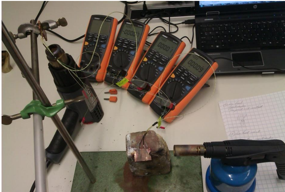
Figure 36: Photo of the experimental setup. The paint dryer and the gas burner are used for temperature control of the copper blocks and three voltmeters are used to record the voltage. The support structures are electrically insulated.
