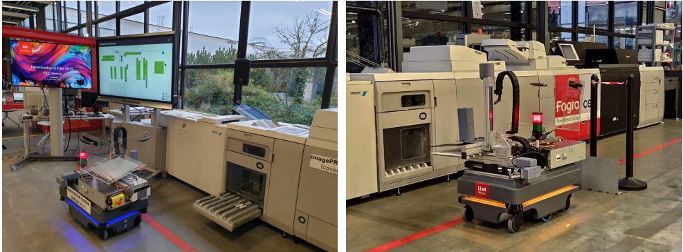
Figure 151: AGV with motorized robot arm and deposit tray for media unloading and transportation, in front of a cover printer.
