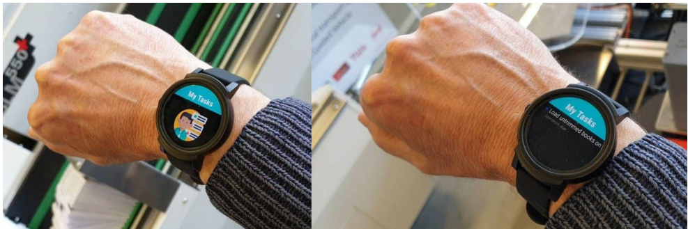
Figure 152: Smartwatch tasklist application for human operators.
