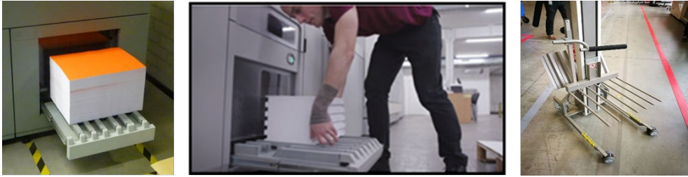
Figure 43: Unloading paper from printers, either completely by hand, or assisted with a forklift (source: OEDIPUS project's material).
