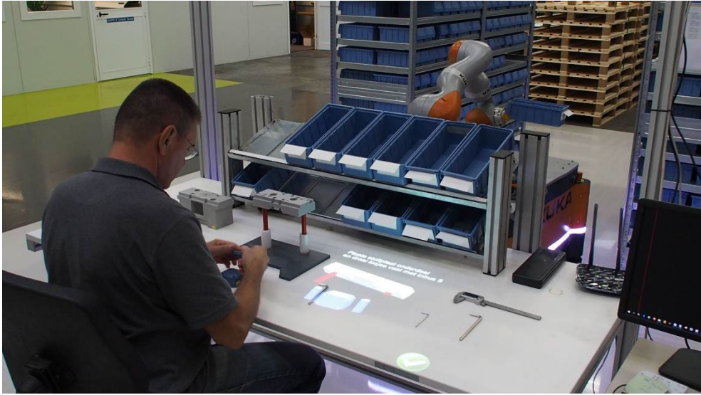
Figure 142: Single tool assembly process at TRI with AR support for assembly instructions and mobile robot for tool parts collection.
