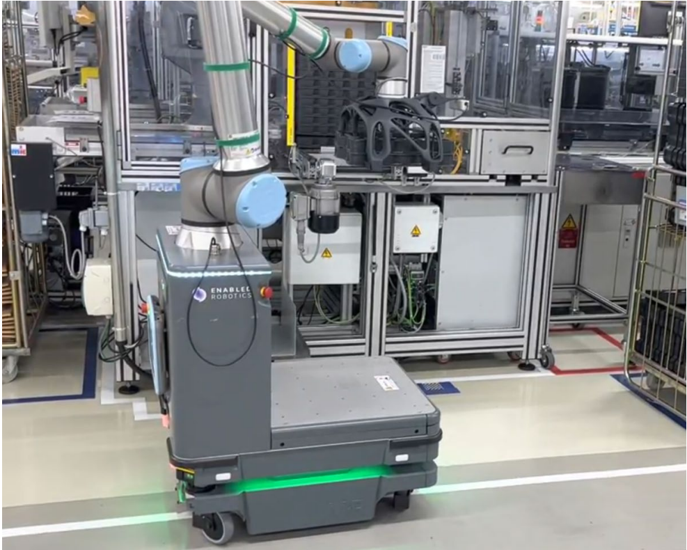
Figure 158: Mobile robot (AGV with mounted robot arm with gripper) feeding empty trays on loading station at BOS.
