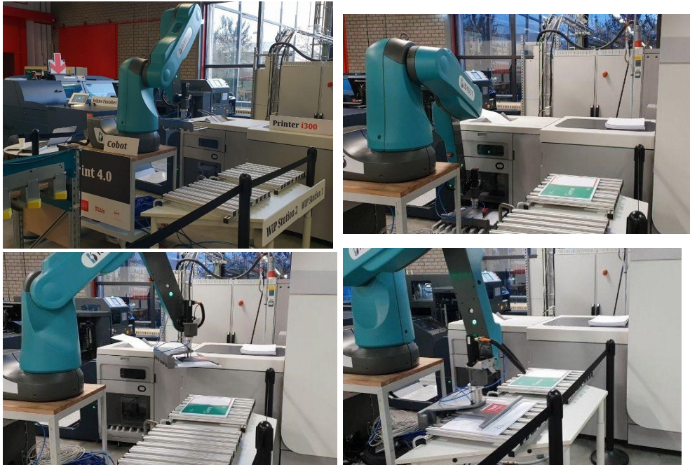
Figure 150: Media unload from printer by a collaborative robot arm 89 .
