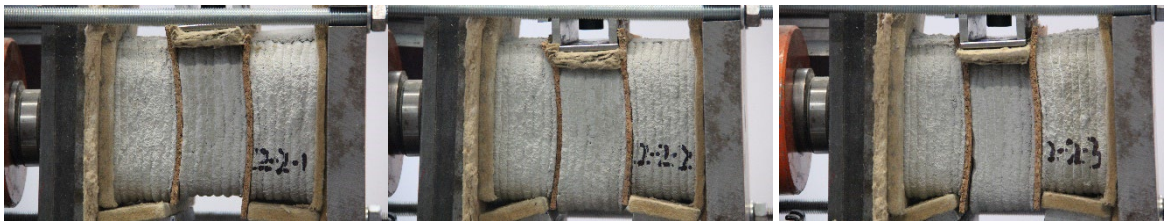
Figure 7-5: The shear test for half sine shape with cork board as interlayer material.
