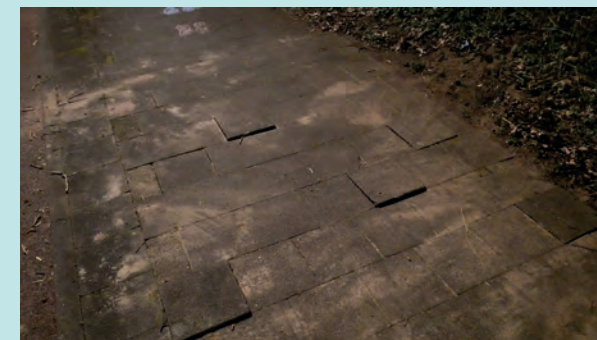
(2) With a hydraulic system it is possible to move different paving stones up and down (obstacles) to simulate unevenness in the footpath
