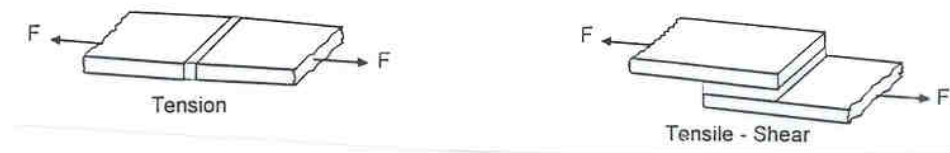
Fig. 9: Adhesive joint design. Left figure not suitable. Right figure typical adhesive joint design.
