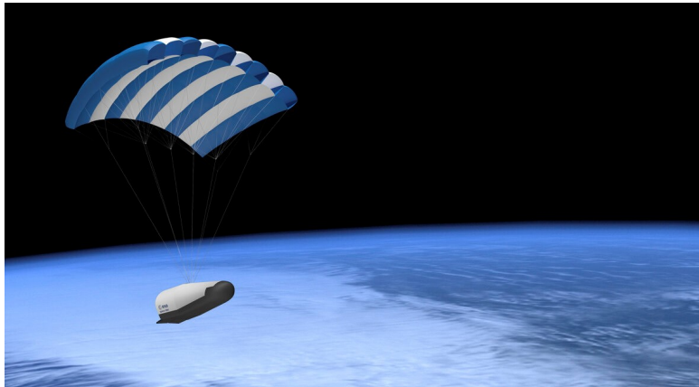
Figure 1: The Space Rider guided by a parafoil
