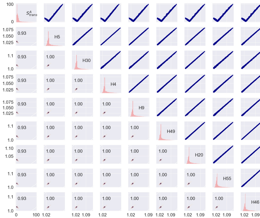
Figure B.2: A pair plot for the transformer phase A loading ( S_{trans}^A ) and voltage magnitudes ( V ) at the POC of the houses H5, H30, H4, H9, H49, H20, H55, and H46 connecting to the same phase. This pair plot consists of histogram plots along the diagonal, Pearson correlation coefficients below the diagonal, and scatter plots above it.
