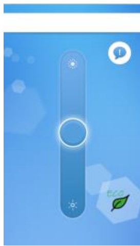
Figure 35. The user interface for controlling luminaires output used in experiment2.
