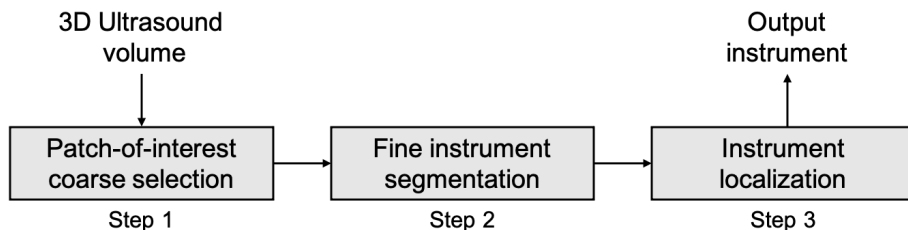
Figure 6.1 Diagram of a coarse-to-fine instrument localization and segmentation system. The diagram has a similar structure as in the previous chapter, but the training methods are different, and also the localization in the first stage is modified.
