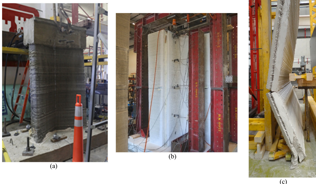
Fig. 4. a–c. Large scale testing: (a) B-Hut wall element, (b) Milestone wall type B element, (c) Beckum House wall.
