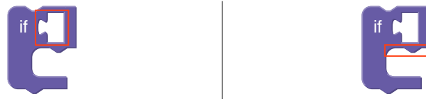
Figure 7.4: If block that highlights the usage of an input value block (left) as its first argument (condition of the if statement) and a statement input (right) as its second argument (body of the if statement).
