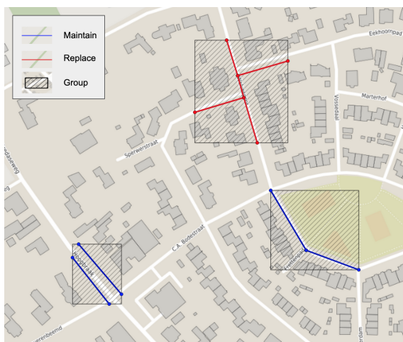
Figure 4: Example of a grouping of interventions on pipes that are close to each other, produced by the DRL+GCN approach for year 50 of the maintenance plan.
