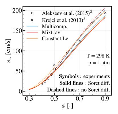
The figure at the left shows that the laminar flame speed of 1D premixed and lean  $H_2$ /air flames is well predicted by all the transport models and the reaction mechanism proposed by Burke et al. (2012)<sup>4</sup> when Soret diffusion is taken into account.
