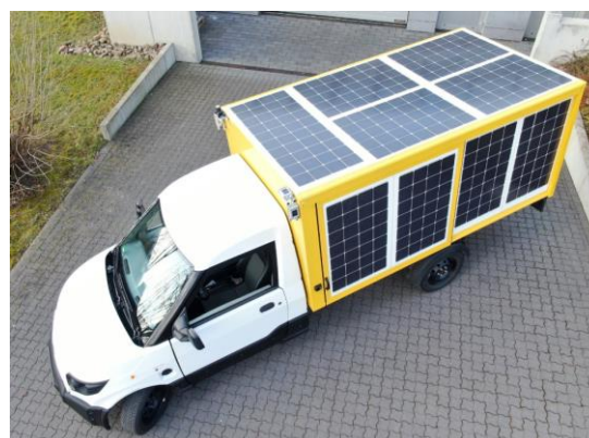
Fig. 2.3-7 PV-powered light commercial vehicle, developed by the Street project (Photo: Institute for Solar Energy Research Hamelin)
