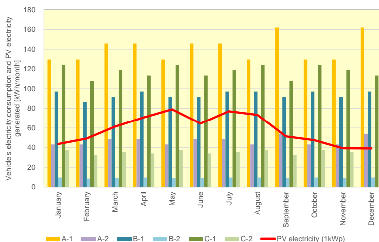
Fig. 2.1-10 Vehicle’s electricity consumption and PV electricity generated
