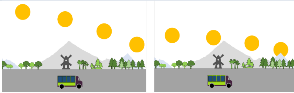
Fig. 2.5-5 Effect of surroundings on the performance of PV panels on trailers (left: high elevation angle, right: low elevation angle)
