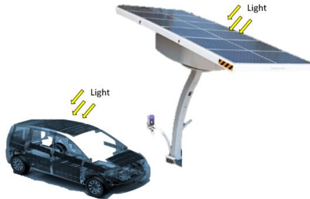
Fig. 4.3-13 PV canopy infrastructure enhanced for PV-powered vehicle
