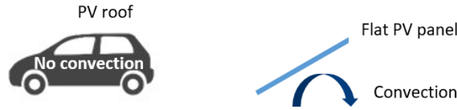
Fig. 4.3-6 Illustration of the convention situations for a built-in VIPV application and a solar PV panel in a rack-mounted system configuration
