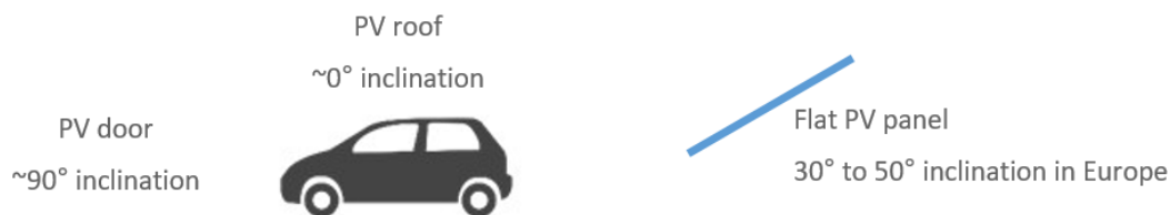
Fig. 4.3-1 Illustration of a PV roof orientation and PV door orientation (on the left) compared to a flat PV panel inclination in a power plant (on the right)
