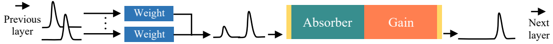
Figure 1: Block diagram of an optical neuron in an SNN, consisting of weighed input pulses injected into the laser
