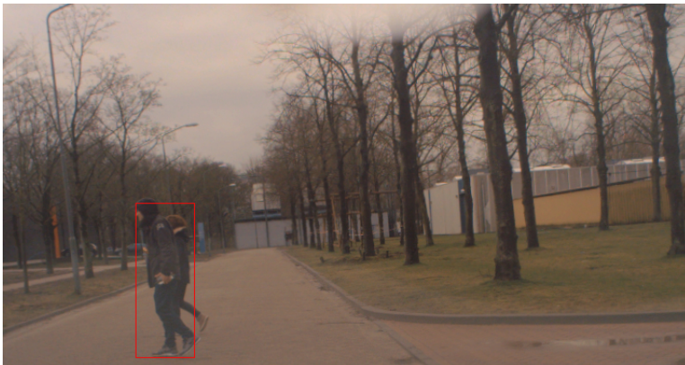
Figure 4.4: One pedestrian occludes another pedestrian. Therefore camera is not able to detect one of them, while both of them have IoT devices.
