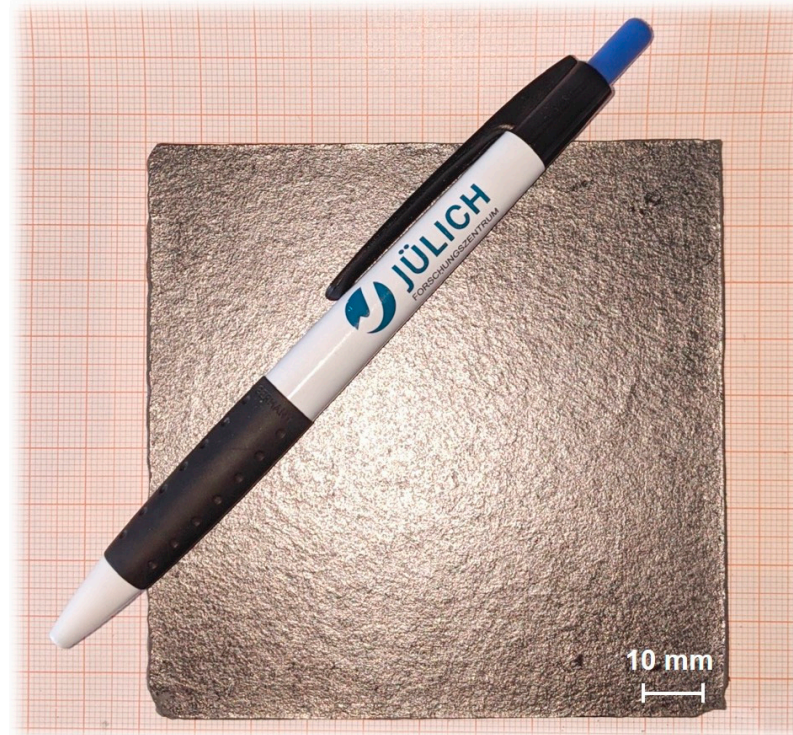
Figure 6. A large-scale bulk SMART alloy sample sintered using the industrial FAST facility.
