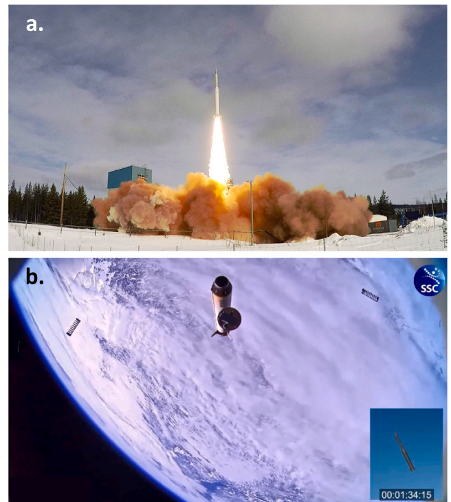
Fig. 7. MAXUS-9 flight: (a) Launch of the rocket from the Esrange site (credit: Neil Melville), (b) separation of the Castor IV rocket booster (long cylindrical section) and of the SUPERMAX parachute testing module (circular object in front), with a view of spring-loaded bolts (upper left and right). The picture is a still image from the Swedish Space Corporation (SSC) video taken by a camera placed on the bottom of the rocket payload (courtesy of SSC).
