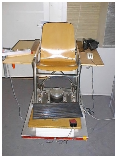
Figure 4: The chair with a scalometer positioned at the right side of the participants.
