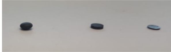
Figure 4.6.: Particles used for single-particle levitation experiments. From left to right a 1:2 oblate spheroid ( p_1 ), a 1:5 disk ( p_2 ), and a 1:10 disk ( p_3 ). All three particles are made of PVC-U.
