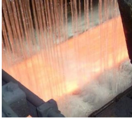
Figure 1.1: Run Out Table in TATA Steel IJmuiden. Moving, red hot steel slab and impinging water jets.
