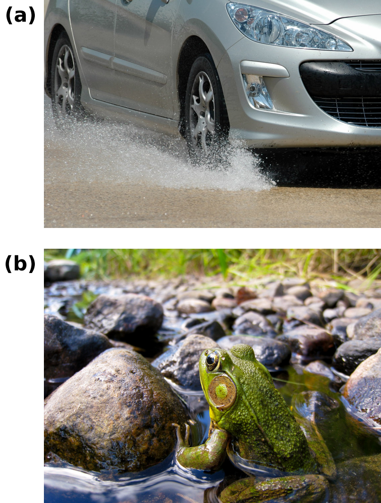
Figure 1.1: (a) A car will slip if a water film forms between the tires and asphalt, causing aquaplaning. (b) A frog can stick to wet and underwater rocks, even in strong currents. “Cours - Kurse - Aquaplaning” by Touring Club Suisse/Schweiz/Svizzero TCS (a) and “Froggy” by Stephen Begin (b) are licensed under CC BY-NC-SA 2.0. To view a copy of this license, visit https://creativecommons.org/licenses/by-nc-sa/2.0/
