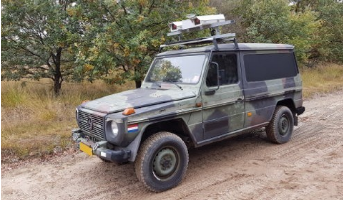
Figure 6.2 — Prototype vehicle with the stereo camera system on top.
