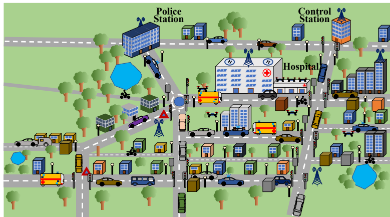
Fig. 1. The urban environment of a future city where all the infrastructure is 5G enabled. Vehicles are fully autonomous and receive signals from lamp posts, traffic lights and base stations throughout the city. The lamp posts also enable 5G broadband wireless access. The control station is responsible for the management of all public infrastructures, including communications and traffic.
