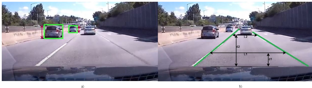
Figure 30: Width Based Methods: a) Intervehicle distance calculation based on bounding box height change b) Intervehicle distance calculation based on lane-markings
