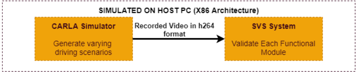
Figure 43: CARLA Simulator setup for unit testing of SVS functions
