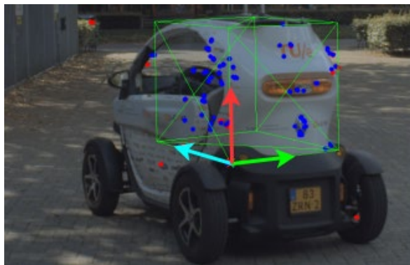
Figure 42: 3D Box mesh manually aligned with the Twizy rear surface and feature points extracted
