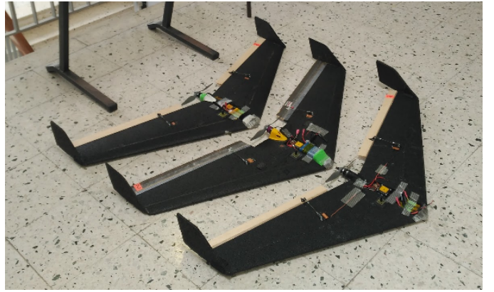
Fig. 4: The three fixed-wing UAVs employed in the experiments. They have a 120cm wingspan and weight around 800grams. The vehicles are powered by the open-source autopilot Paparazzi .
