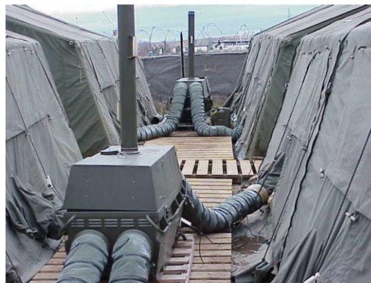
Figure 7 Mobile heater, Dantherm VA-M 40
