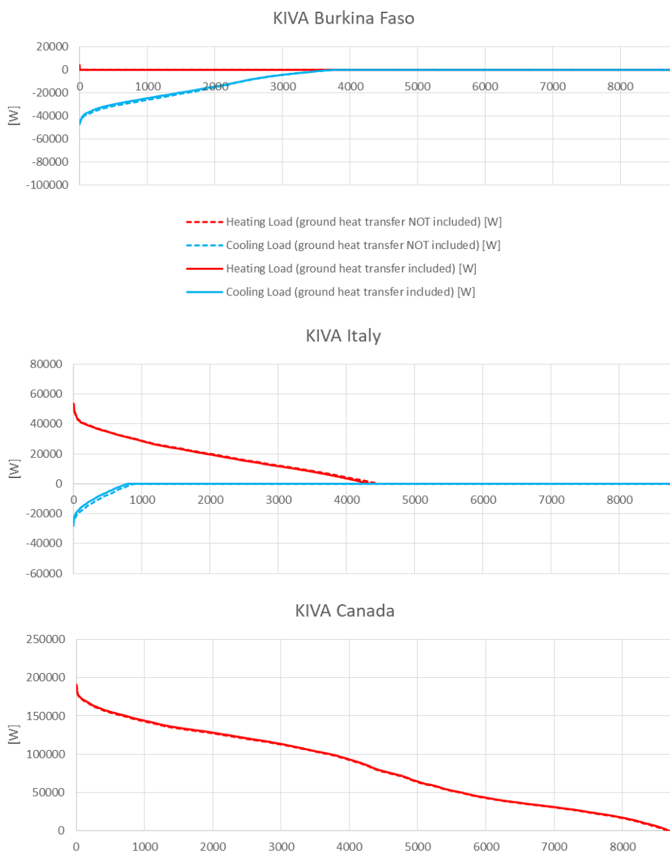
Figure 19 Load duration curves calculated using the Kiva ground modeling method
