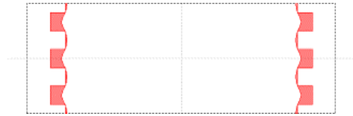
Figure 5.5: Resulting mismatch polygon by performing XOR logical operation on design intent and simulated resist pattern.
