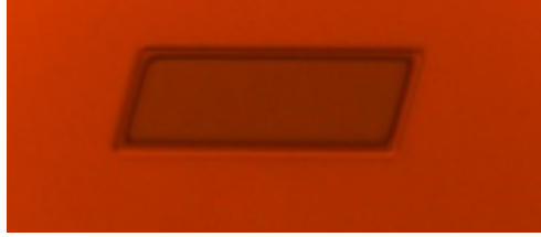
Figure 3.3: Example of ArF resist under-etch after BHF hard mask etching prior to cleaning.
