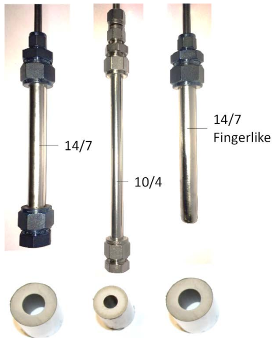
Figure 2.1. Sealed membranes with a cross-section; from left to right: a 14/7 mm OD/ID membrane, a 10/4 mm OD/ID membrane and a 14/7 mm OD/ID finger-like membrane.
