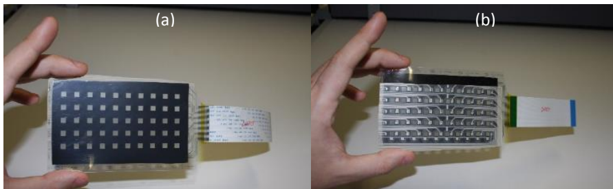
Figure 80. Proximity sensing surface obtained after lamination process. (a) Front view. (b) Back view
