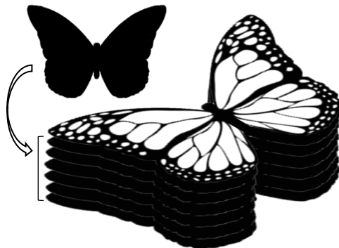
Figure 5.2: Schematic drawing separating the layers of the 3D printed butterfly. All layers except the final layer are completely filled with the printed polymer. In the final layer, only the veins and contour of the butterfly were printed (black), serving as the walls, leaving the white areas in the wings open to be filled with ink.
