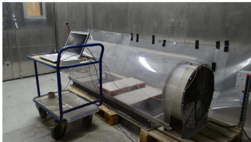
Figure 4: Wind channel with four previously plastered paving slabs (30 x 30 cm) in a climate chamber operated at 30° C and 50 % relative humidity
