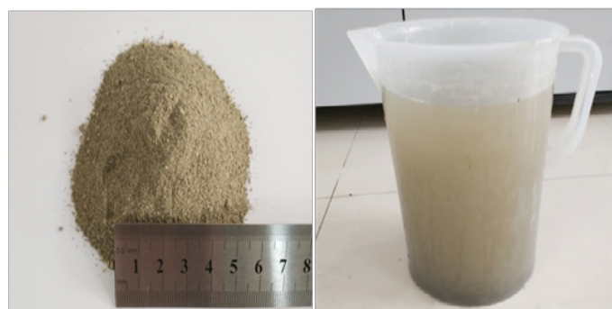
Figure 3: a) Clogging material mixed by sand and dredged silt, b) The suspension of clogging material has a concentration of 1%.
