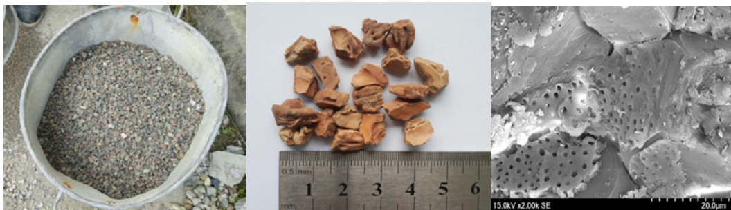
Figure 1: a) Normal weight aggregate, b) Crushed peach shell and (c) SEM image of peach shell.
