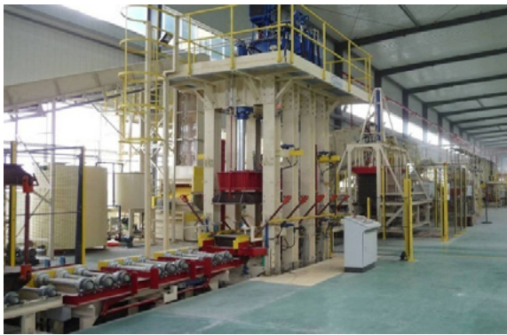
Figure 10 - WSCB Plant with EltoBoard Press Figure 11 - WSCB applied in walls, floors and roof (Takemura, Japan)
