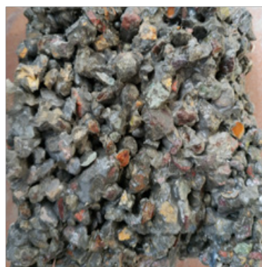
Figure 6: Failure pattern of PC containing PS.
