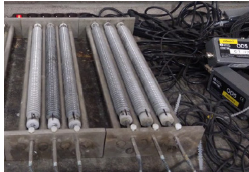
Figure 2: Set up for the autogenous shrinkage measurement.
