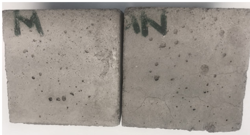
Figure 6: Physical outlook appearance of both mortars after 56 days; Left: CN-LSG (NW) and Right: SCN-LSG (W).
